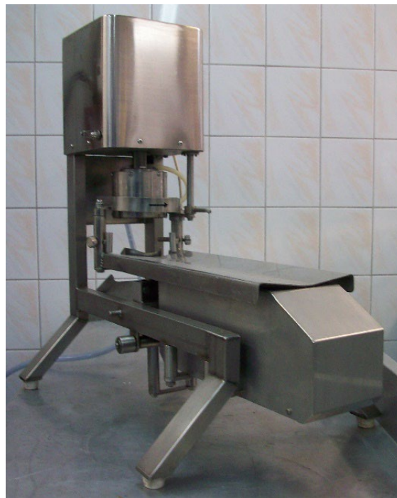
Fig. 2. Deheader for carp with a circular cut (prototype)
