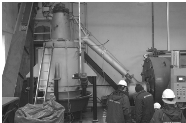
Fig. 1. The counter-current gasifier used in the experiment
