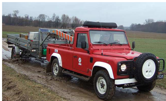
Fig. 6. Land Rover Defender coupled with gooseneck trailer during field tests
