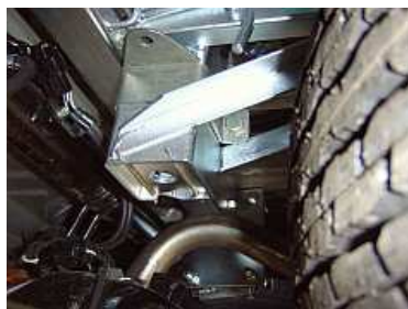
Fig. 11. Side view of hitch ball support frame
