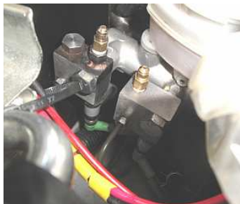
Fig. 28. Mitsubishi L200 – two hydraulic pressure transmitters mounted under special connectors on brake pump. On top visible air bleeding valves
