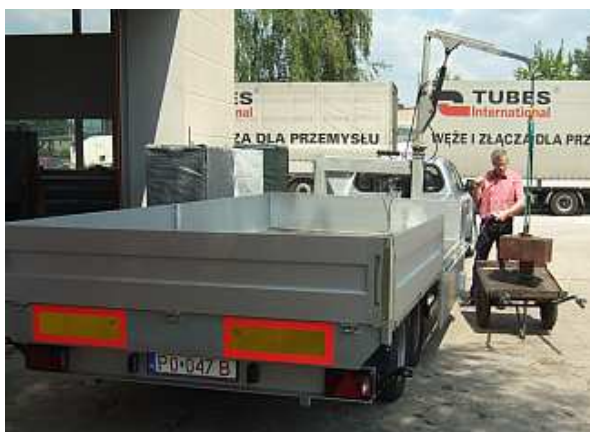
Fig. 20. Tests of unloading 200kg weight, behind gooseneck trailer visible forestry containers with agrotexile canvas cover (green, white, black, silver as on trucks)
