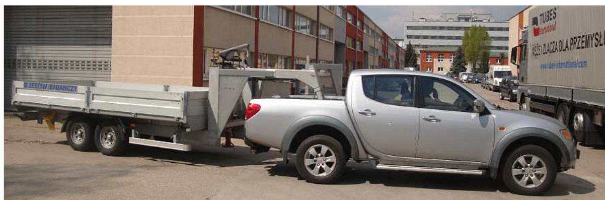
Fig. 13. Mitsubishi L200 truck with gooseneck trailer and collapsible hydraulic lift for unloading containers with small trees from forestry nursery
