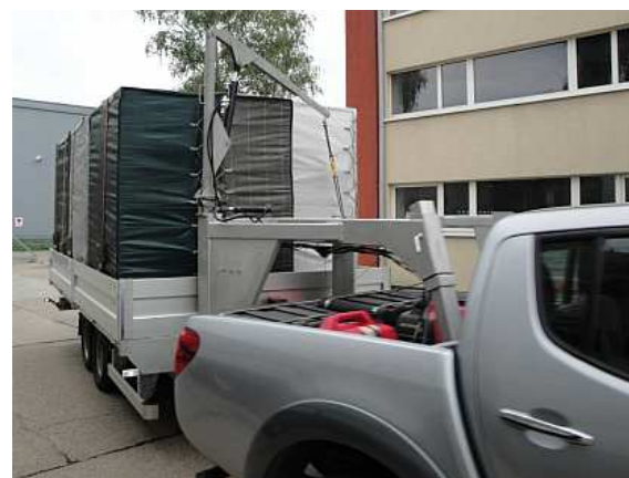
Fig. 21. Gooseneck trailer loaded with 9 containers for transportation of small trees from forestry nursery
