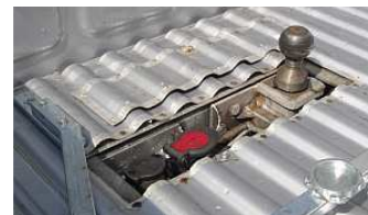
Fig. 9. Hitch ball in working position and sockets
