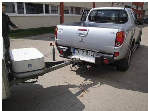
Fig. 31. L200 truck coupled with trailer - PEBS is mounted under white cover
