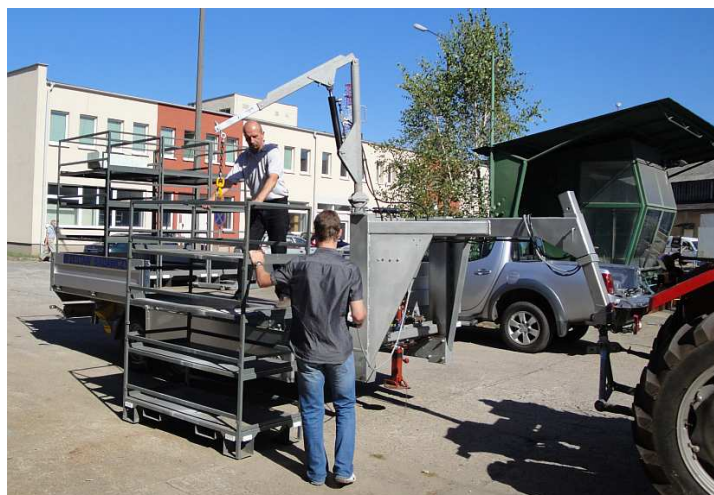
Fig. 27. Farm tractor coupled with gooseneck trailer - functional tests of unloading system
