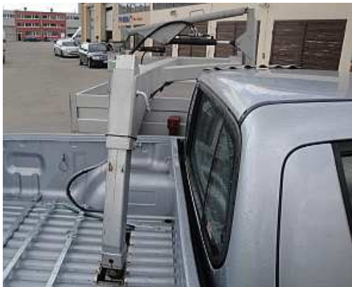
Fig. 22. Special tongue frame design allows for tight turns of gooseneck trailer
