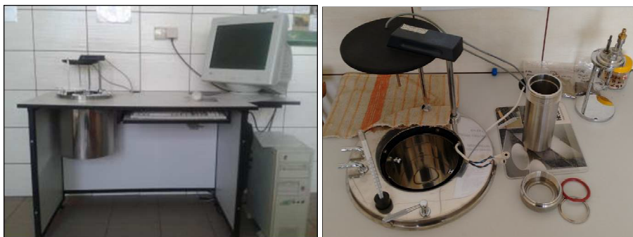
Fig. 2. Computer Calorimeter KL-12Mn2 (on the left), general view of the test stand (on the right)
