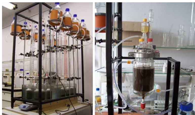
Fig. 3. Research stand for the study of biogas productivity of substrates according to DIN 38414 s.8 (on the left), inoculum station for quasi-continuous fermentation work (on the right)
