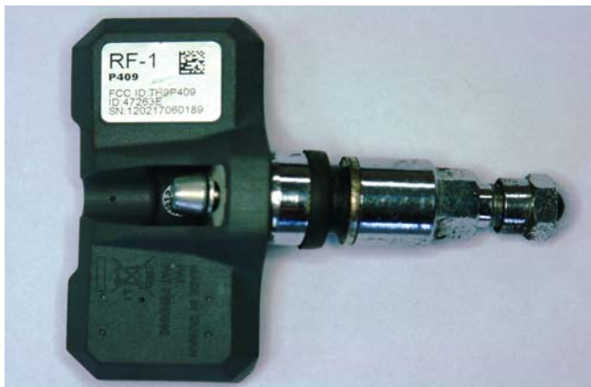
Fig. 1. TPMS P409 sensor (433,92 MHz) Rys. 1. Czujnik TPMS P409 (433,92 MHz)
