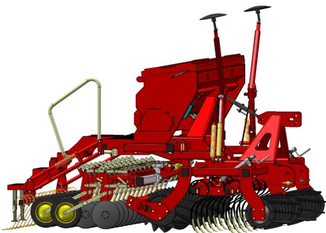
Fig. 1. The model of tilling-and-sowing combined machine Rys. 1. Model agregatu uprawowo-siewnego
