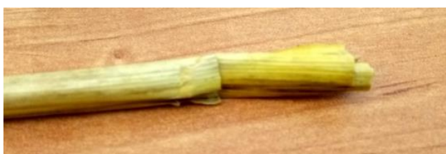
Fig. 16. An example of moisturized sample which was not separated during a test at gap width 0,2 mm and cutting speed 2 \text{ mm} \cdot \text{s}^{-1}
