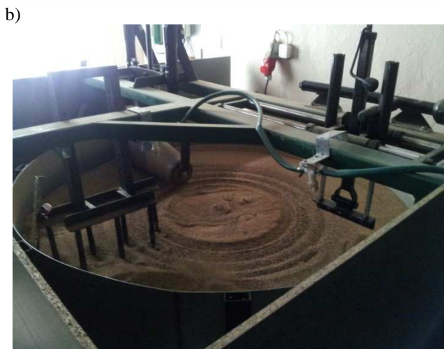
Fig. 2. The „rotating bowl” unit: a) scheme [5]: 1 - transmission, 2 - engine, 3 - running rail, 4 - bowl, 5 - holder of the sample, 6 - supporting frame, 7 - roller: 8 - frame of the bowl, 9 - main frame, b) view [6]
