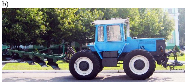
Fig. 1. Ploughing aggregates, created according to the schemes \langle 2+4 \rangle (a) and \langle 0+5 \rangle (b)
