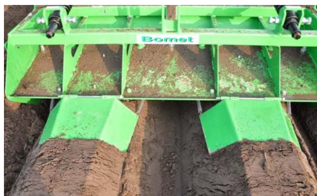
Fig. 5. Cover plates forming ridges [3]
