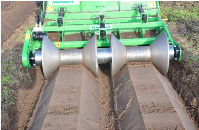
Fig. 7. Ridges formed by spool shaft [3]
