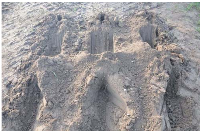
Fig. 3. Working tracks of 3 passive teeth, knives of active milling drum and ridging corps [3]
