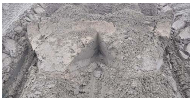
Fig. 6. Working tracks of 2 passive teeth, knives of active milling drum and ridging corps [3]
