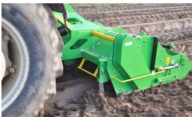
Fig. 4. Passive tooth behind the wheel of the tractor [3]
