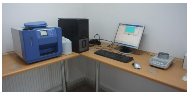
Fig. 2. Test stand for determining the higher and lower heat value
