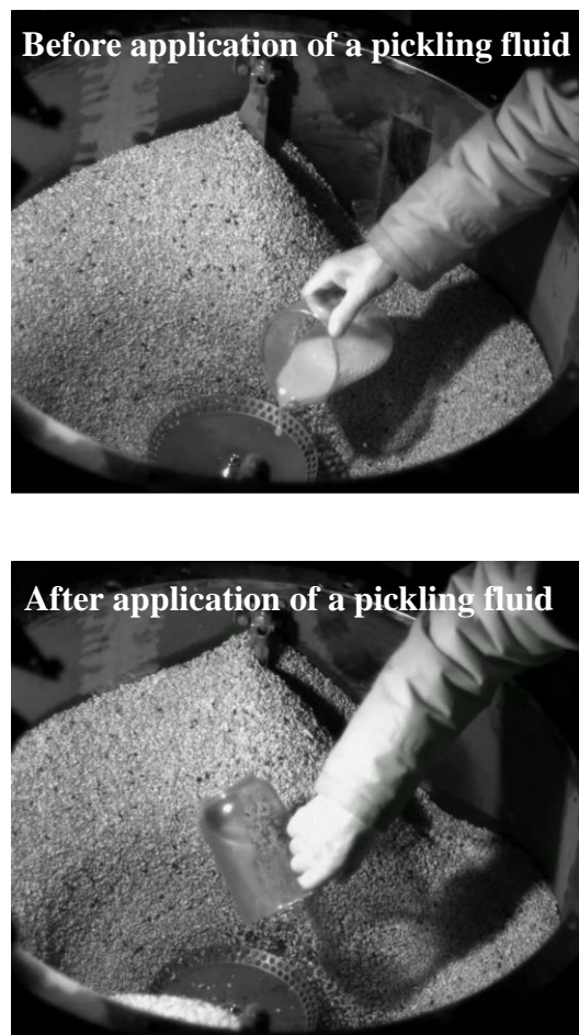
Fig. 7. Seed distribution and range of grain on the internal surface of the working chamber depending on the presence of seed pickling fluid during operation with scraping elements for supply current frequency 35 Hz
