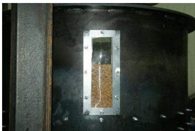
Fig. 1. Observation window in the seed pickling machine on the side wall
