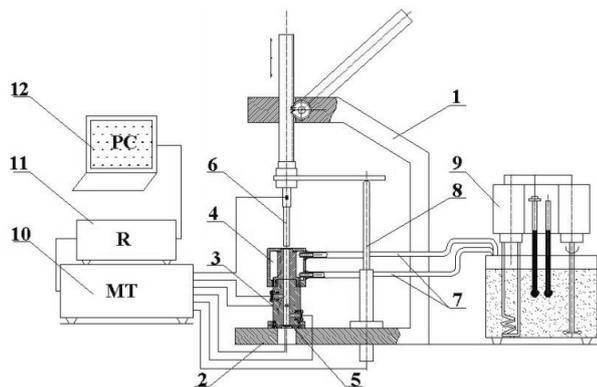
Fig. 1. Scheme of the SS-3 test stand for testing the agglomeration process [16]: 1 - press, 2 - base, 3 - compaction chamber, 4 - thermostatic element, 5 - chamber bottom, 6 - compacting piston, 7 - stub pipes, 8 - displacement sensor, 9 - ultrathermostat, 10 - strain gauge bridge, 11 multi-channel recorder, 12 - computer
