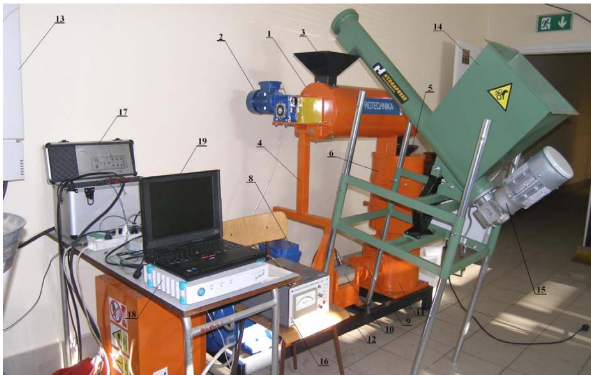
Fig. 1. Working stand with a new prototype pelleting and briquetting device with a flat immovable matrix [5, 13]: a) scheme of the stand: 1- mixing-pelleting-feeding system, 2- drive of the mixing-pelleting-feeding system (electric motor connected with a reducer), 3- raw material inlet to the mixing-pelleting-feeding system, 4- mounting frame of the mixing-pelleting-feeding system, 5- raw material inlet to the working system of the pellet mill, 6- working system of the pellet mill, 7- outlet of pellets from the working system, 8- drive of the pellet mill (electric motor), 9- clutch, 10-Mi20 torque measuring shaft, 11- spur gear, 12- base, 13-frequency converter, 14- feeder, 15- feeder drive (electric motor connected with a reducer), 16- WT-1 torque and force indicator, 17- METROL KWS 1083 device for active power measurement, 18- Spider 8 recorder, 19- PC computer; b) view of the stand
