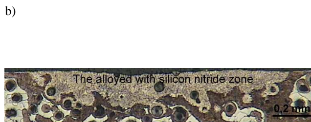
Fig. 2. The surface layer microstructure of cast iron after laser alloying with silicon nitride with laser beam power: P = 2600 W (a) and P = 330 W (b). Optical microscope
