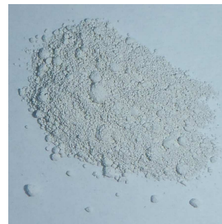
Fig. 1. \text{Si}_3\text{N}_4 powder applied during laser heat treatment
