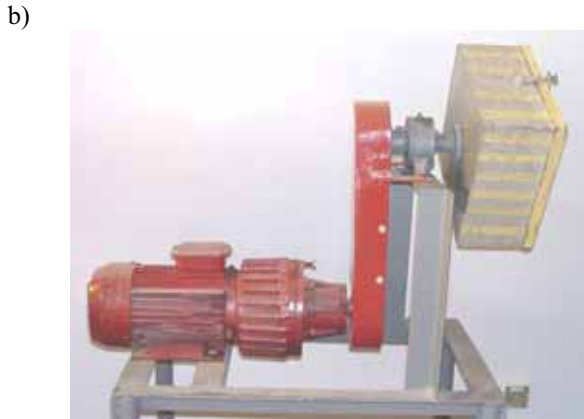
Fig. 5. Stand for the measurement of coefficient of kinetic durability P_{dx} of pellets using Prost's method: a) scheme of the stand: 1 - frequency converter, 2 - electric motor, 3 - belt transmission, 4 - tester chamber, b) stand view
