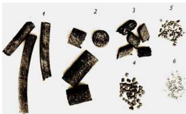
Fig. 1. Example: pellets (4, 5, 6 – a diameter of 4; 6,5; 8,5 mm; briquettes (1, 2, 3 – a diameter of 28 mm, 50 mm) from biomass [2, 3]
