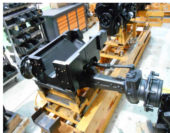
Fig. 1. D4CS4-FA20.25 front axle bracket of URSUS C-380M tractor with a mounted axle
