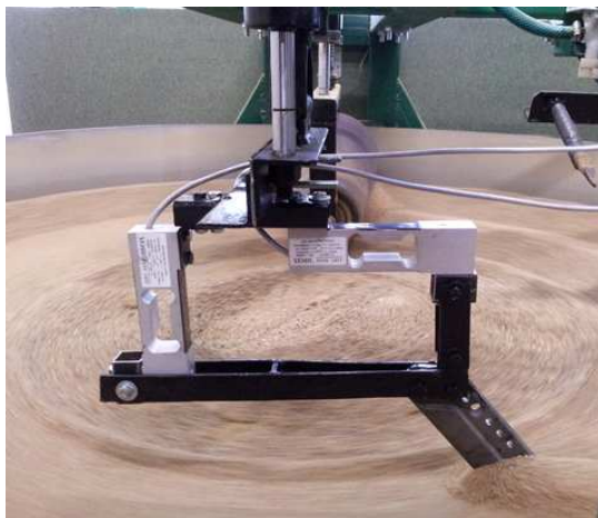
Fig. 4. The measuring system used to measure the force on the hoe coulter [9]
