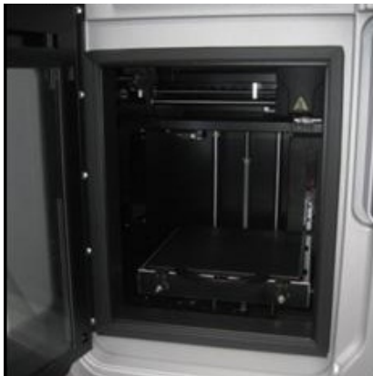
Fig. 5. 3D Printer Stratasys Dimension 1200es – work chamber
