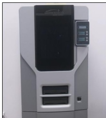
Fig. 4. 3D Printer Stratasys Dimension 1200es Rys. 4. Drukarka 3D FDM Stratasys Dimension 1200es
