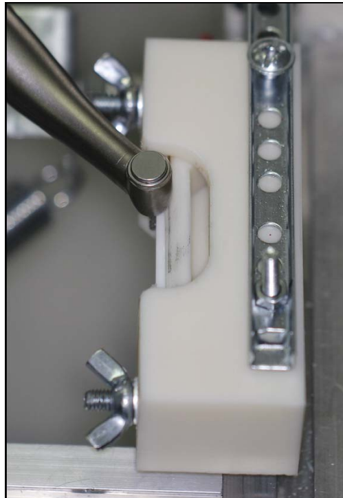
Fig. 7. Test sample mounting with fixed sample prepared for testing
