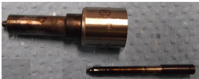
Fig. 10. Nozzle - there are visible signs of strong overheating of the nozzle in the form of brown discoloration, which caused seizure of the needle and blockage of the fuel flow [16]
