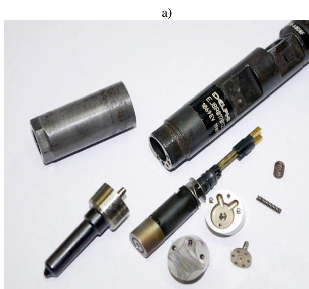
Fig. 12. Components of the injector (a), damaged coil of the piezo injector (clear traces of corrosion and loss of material caused by water entering the coil through leaking seals (b) [16]
