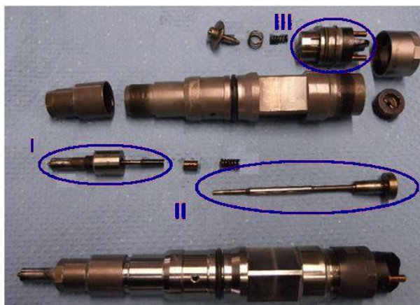
Fig. 4. Components of Common Rail electromagnetic injectors subject to wear, where: I – nozzle, II – needle valve, III – solenoid assembly with armature
