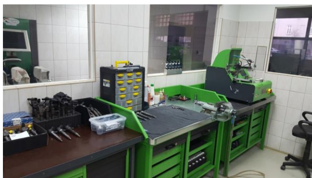
Fig. 16. Test bench for injectors with the EPS-200 tool from Bosch [10]
