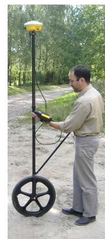
Fig. 1. Set for quantity survey of ditch - GPS stick with wheel and receiver
