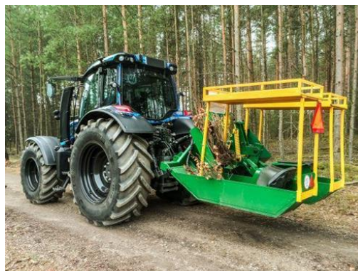
Fig. 4. Construction of the RZS-2 planter mounted on a tractor [4]
