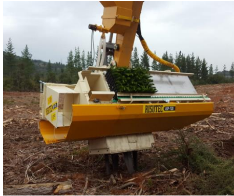
Fig. 5. The structure of the Risutec ASP-720 planting device suspended on the arm of a tracked excavator [5]
