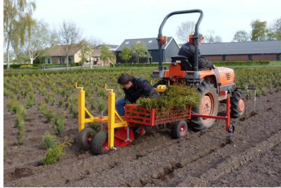
Fig. 3. Damcon brand structure, mounted on the rear linkage of the tractor, single-row version [3]
