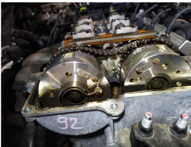
Fig. 6. Damaged timing system in Kia Sportage 1.6 TGDI engine Source: (Author's own work)
