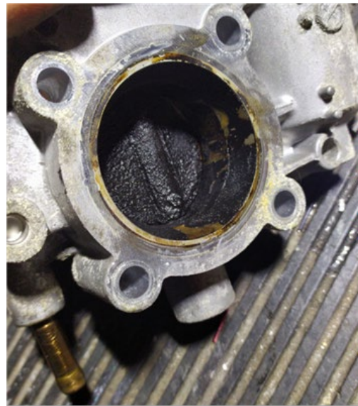
Fig. 4. Contaminated engine throttle. Source: (Author's own work)
