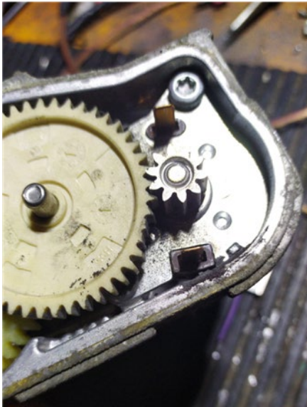
Fig. 3. Hyundai Tucson 1.7 CRDI – sheared teeth preventing engine operation. Source: (Author's own work)
