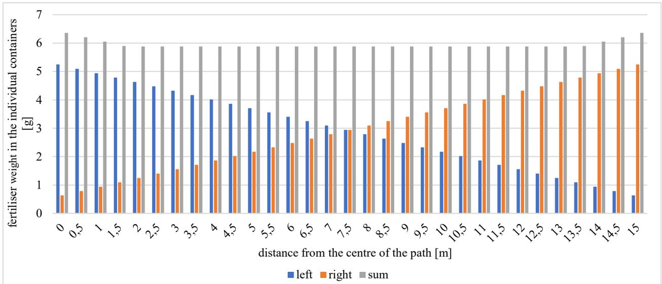
Fig. 3. Total fertiliser weight as a function of the distance between two passes of the Unia Brzeg 850MX spreader
