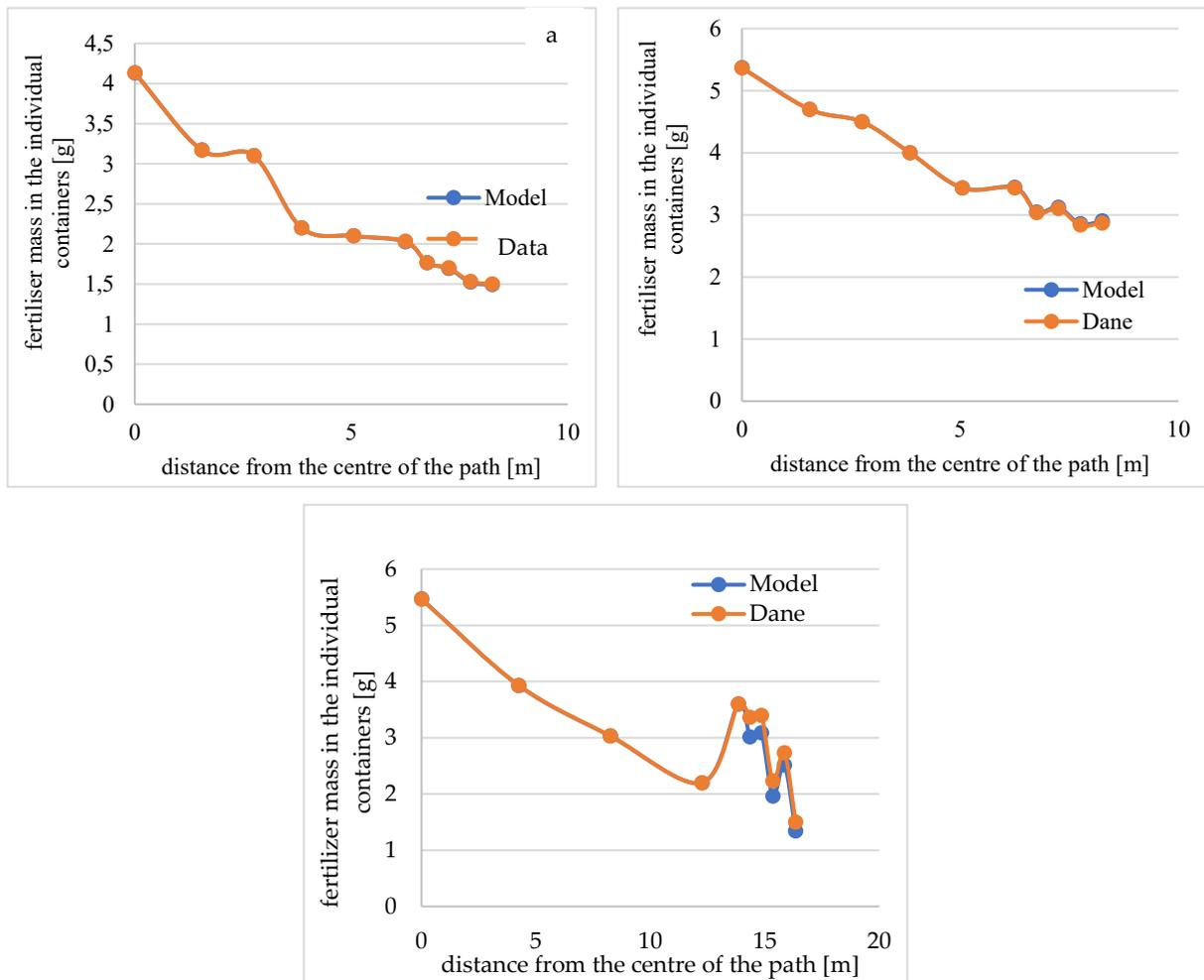
**Fig. 5.** Graph showing the goodness of fit of the constructed model to the experimental data for a. Amazone spreader, b. Unia Brzeg 850MX spreader, c. Kuhn Rauch Axis 30.1EMC.W spreader
