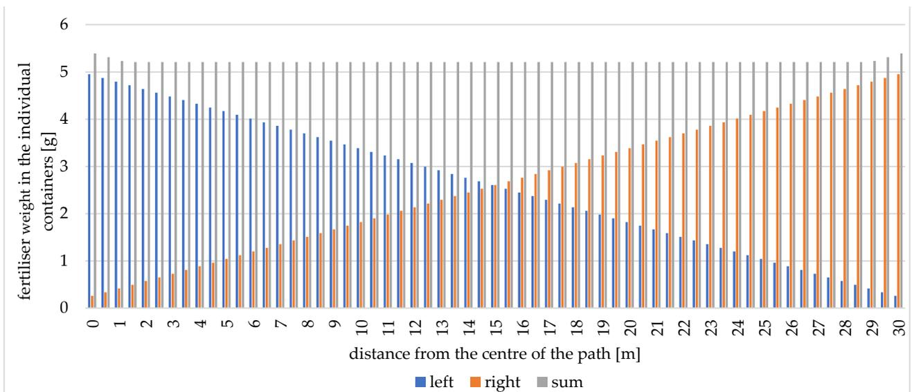
Fig. 4. Total fertiliser weight as a function of the distance between two passes of the Kuhn Rauch Axis 30.1EMC.W spreader
