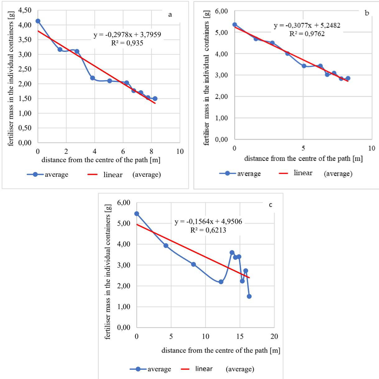
**Fig. 1.** Fertiliser weight as a function of distance from the spreader axis perpendicular to the direction of movement: a. Amazone, b. Unia, c. Kuhn spreader
