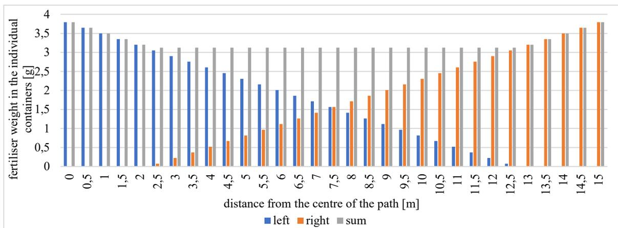
**Fig. 2.** Total fertiliser weight as a function of the distance between two passes of the Amazone ZA-M spreader
